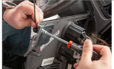
2. Line up the pedestal and the backing plate with the drilled holes. Secure in place using the enclosed screws and locking nuts.
