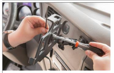
4. If you prefer NOT to use the Tilt-Swivel remove it by undoing the four screws on the face of the cradle. Then mount the cradle directly to the pedestal. (screws for mounting the cradle directly are not included and will need to be obtained separately)
